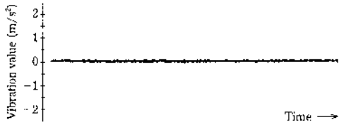
Fig. 1 Original wave form of the normal bearing
